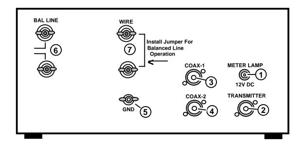
*1. Meter Lamp:* 2.1-mm coaxial power jack accepts 12 vdc to operate the LED meter lamps and the metering circuit (see text)
