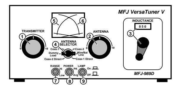
1.) **Transmitter Tuning Capacitor:** Series capacitor on the *Transmitter* side of the T-network. Maximum capacity at  $\underline{0}$  knob setting and minimum capacity at  $\underline{10}$ .\*
