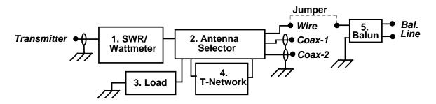
1.) **SWR / Wattmeter:** Dual-range (300W/3kW) power meter features precision cross-needle movements with LED illumination, a compensated directional coupler, and dual detectors for measuring average and instantaneous-peak power. Circuit is identical to our MFJ-815C *TrueActive* (TM) standalone meter.
