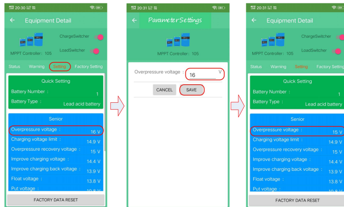
Figure 5-5 Parameter setting - overvoltage voltage setting
