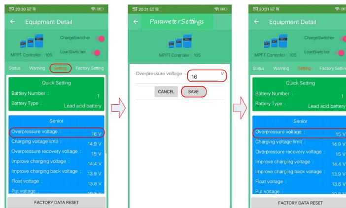
Figure 4-5 Parameter setting - overvoltage voltage setting
