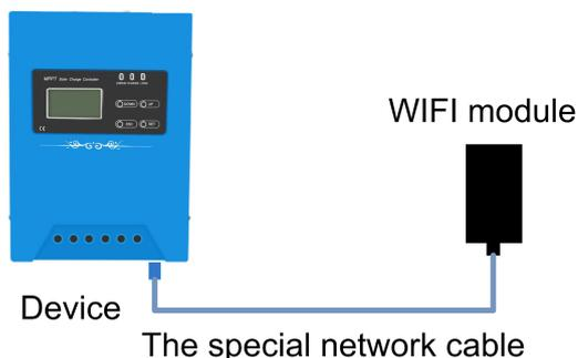
Figure 2-3 Connection diagram between the device and the WIFI module
