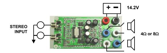
Figure 1: EB-TA2021B Rev.D Connections
