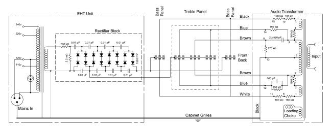
Figure 3: Quad ESL Schematic Diagram
