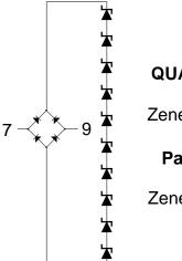
QUAD Parts: Diodes: GP02-30 Zener Diodes: BZT03C220
