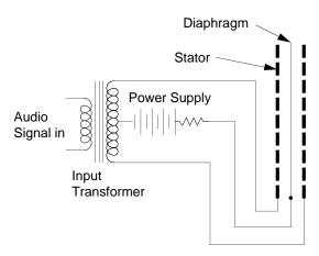
Figure 1: ESL electrical diagram
