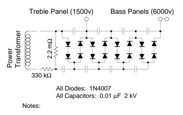
When bolting circuit board to power supply frame, use 1/4" stand-offs to insure that the traces are far enough away from the metal frame to prevent arcing.
