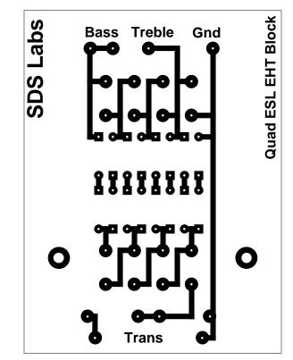
Figure 6: Replacement Rectifier Block Design
