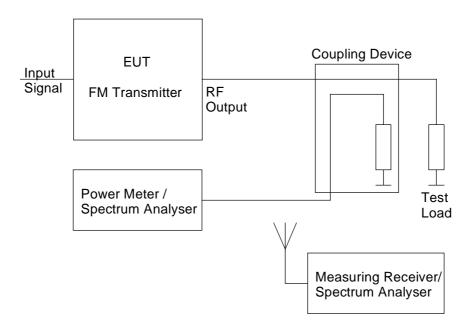
Figure A.5: Testing arrangement for cabinet radiation
