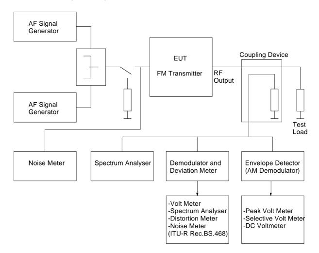
Figure A.1: Testing arrangement for monophonic transmitters
