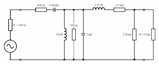
Figure A.4: Filter circuit
