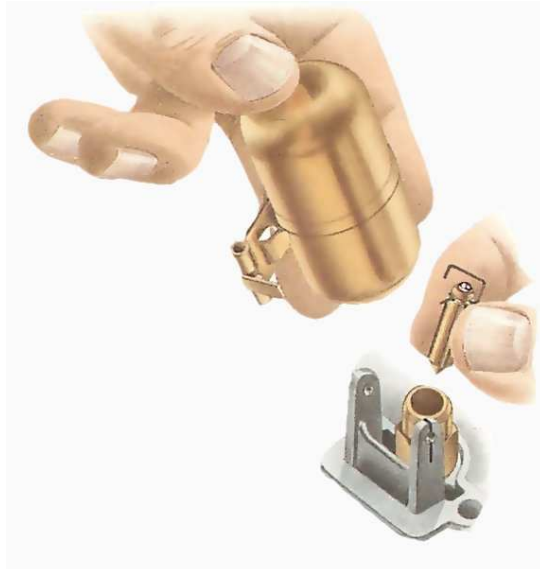
Remove the needle valve for cleaning the valve and its seat.
